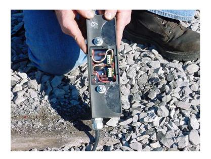
This photo shows a properly wired wheel sensor used in a daisy chain application. A non daisy chain application would have the wires connected to only one connector.
