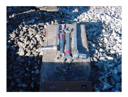
The wrenches required to install the sensor and bracket assembly are 9/16" and 3/4". In addition a Combination Square with a bubble level will be needed to set the height of the wheel sensor.
