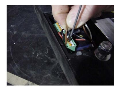
The photo above shows the correct method to remove the wires from the spring cage connector. It is necessary to use a small screwdriver to press in on the small orange tabs located next to each wire installation cavity. Pull on the wire as the tab is pressed in. This will allow the spring cage to release the bite on the wire.
