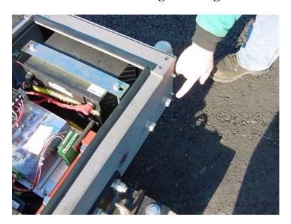
The power and communication cable should be stripped back 24" before inserting the cable through the cord grips. The cable should be pushed through the cord grips until the cable jacket is fully into the cord grip to assure a watertight entrance. Tighten the cord grips after installation of the cable.
