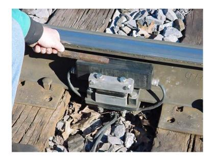
The easiest way to test the Wheel Detection System is to use a railroad spike to "swipe" the wheel sensor. The spike must be held flat and must be swiped over the entire length of the sensor in the direction a train would travel to enter the protected zone to register a valid count on the sensor. This action simulates an axle entering the protected zone and will register a valid count thereby disabling the Switch Machine. This is indicated on the main module by the extinguishing of the # 1 LED.
