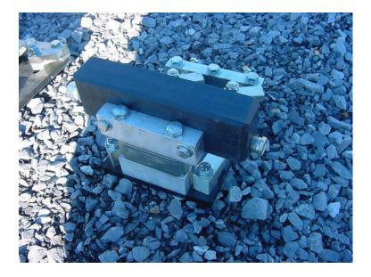
Select the appropriate wheel sensor and bracket assembly for installation at the location prepared to receive the assembly. This photo shows the sensor used at an end of run or for example a single facing point sensor. One end of the sensor has a cord grip to allow the installation of the communication
