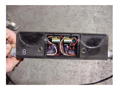
This photo shows correctly installed wires on one side of a wheel sensor that will next be wired in a daisy chain fashion. Notice that none of the connected wires are routed over the orange release buttons on the connectors. This wire arrangement is used typically on the trailing side of the points to connect the reverse wheel sensor with the normal sensor.
