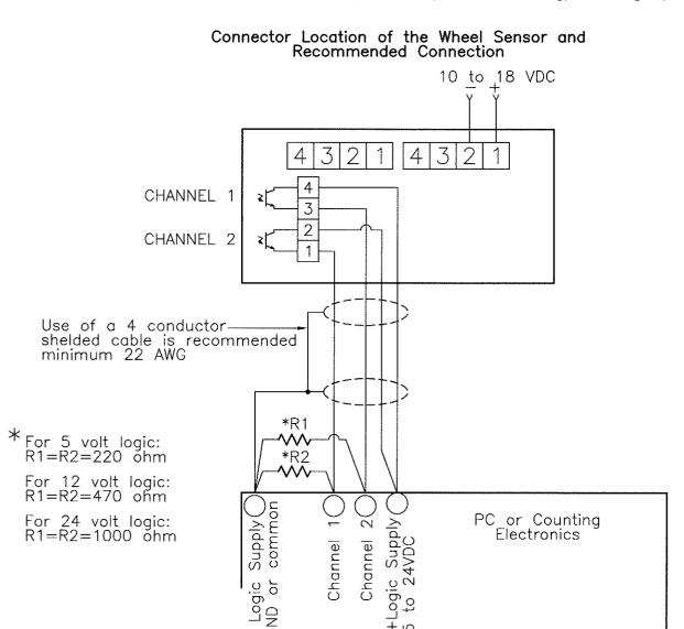
Two channel outputs are provided in Quadrature format with about  $90^{\circ}$  electrical shift as the wheels pass over the sensors.
