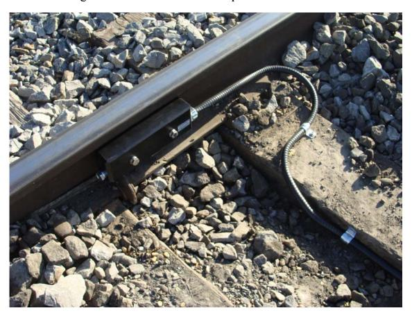
As shown in the above photo, leave enough extra cable so as to allow movement of the rail and re-wiring of wheel sensors in future.
